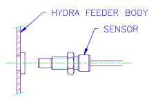
POSITION END OF SENSOR APPROXIMATELY 1/4" FROM MAGNET ON AUGER. TIGHTEN JAM NUT. DO NOT OVER TIGHTEN.
